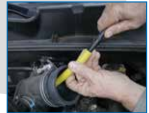
Install appropriate port adaptor and insert smoke solution supply hose into adaptor
